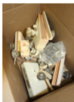
Original crystal doorknobs and mortises, (no longer manufactured) are collected by staff and rebuilt to help maintain original look of building.
